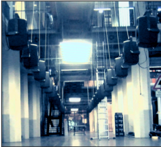
Fig. 2: Auditory-Channel: stereo corridor setup
